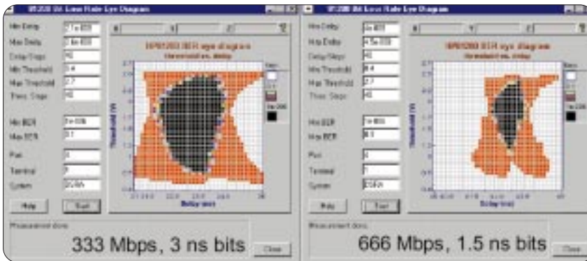
Figure 5. BER eye diagrams for two data rates show how the bit width decreases as the signaling frequency increases.
